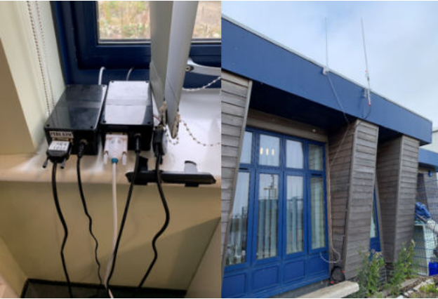
Fig. 1. The AIS receivers and antennas for processing the NCL-DASB dataset which is located on the coastline of Tynemouth port in UK.
